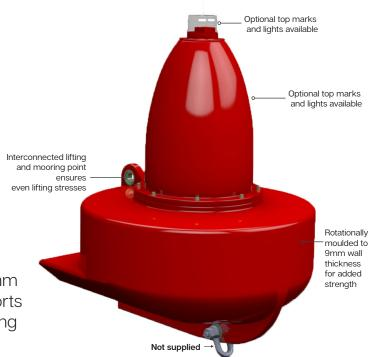
Designed using a traditional navigation buoy shape above the water line and incorporating the shape of a boat hull on the bottom, the SL-B1200-FW remains extremely stable and buoyant in fast and rough conditions. Its unique design incorporating an integrated bow and keel, allows the SL-B1200-FW to create lift as the water flows underneath it, enabling the buoy to rise and sit higher on the surface of the water creating more stability and allowing it to support a heavier payload.
