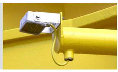
The AL 350 is suitable for lighting objects that cannot be easily located. Coming in two versions (100 or 30 degrees beam angle) and comprising high intensity LEDs, it is powered by an automatic regulating current source with reverse polarity protection. The LEDs and electronics are moulded in an epoxy compound. The light output can be factory set.
