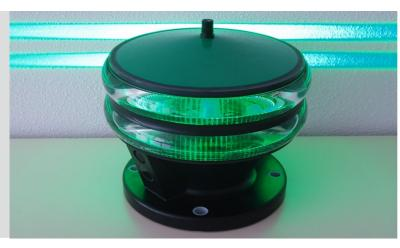
The IML 250 is a ten-mile, advanced LED beacon. The light source comprises high intensity LEDS with precision reflectors and horizontal scattering lenses, which provide consistent horizontal divergence. Housing and top are painted with two layers of high impact polyester powder (signal grey). Provisions are made for air pressure equalisation and to prevent moisture from entering the casing.
