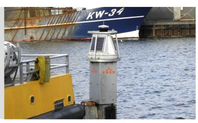
The SPB 300 5 NM is both versatile and costeffective. This five-mile LED beacon is a compact, self-contained solar powered beacon available in red, green, amber, white and black. The lantern is provided with a scattering lens to provide consistent horizontal divergence. The light source is formed by horizontally placed high intensity LEDs. Output can be set according to visibility.
