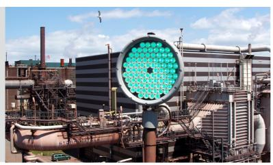
A high intensity leading light for marine signalisation. Different divergence angles can be factory set via filters and reflector adjustments. The light source is formed from high intensity LEDs, each having its own reflector and optics. Light output can be set according to visibility.
